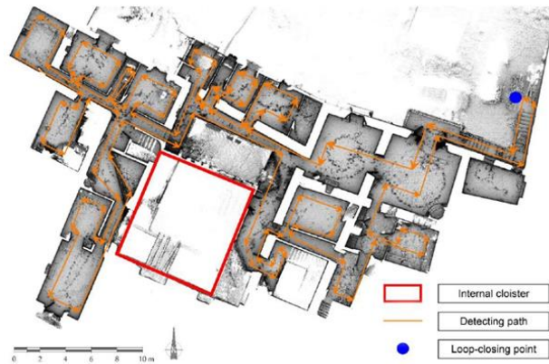
Figure 63. Data collection for indoor scanning: following close-loop protocol for each room scanning
