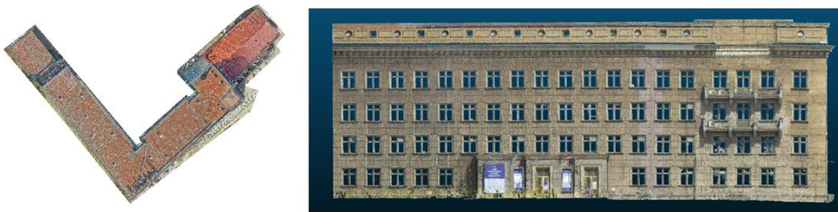
Figure 22. Facade extraction of Pilot project 3
