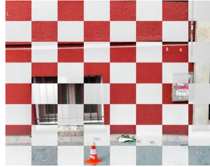
Figure 34. RGB and thermal registration
