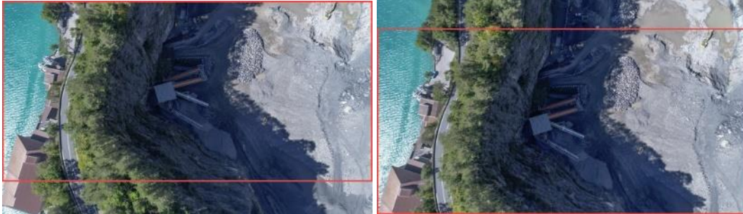
Figure 76. Concept of overlap between images for the 3D reconstruction
